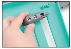
Remove door lock mechanism. Store the lock mechanism & bolts in a safe place for future use.
